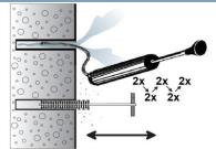
2. Thoroughly clean the hole as follows using a steel- polymer cleaning brush with required extensions and a hand blow pump; 2x blow out drill hole, 2x brush clean, 2x blow out drill hole, 2x brush clean, 2x blow out drill hole.
